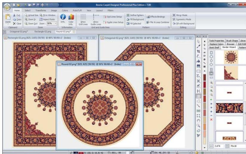
By using **Booria Carpet Weaver** you can convert designs into machine specific production data; supporting, single, double and triple rapier, face to face and incorporate techniques with a large range of weave sets.
